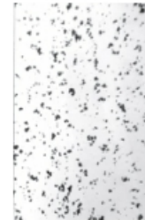
Asphaltenes in the process of precipitating in fuel oil not treated with ADERCO
